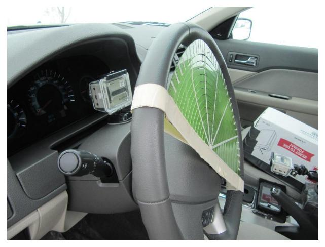
Looking at the above photo you should also be able to see our GoPro22 anchored on top of the steering column in front of the steering rim and pointing at the speedometer, tachometer and other instruments. This arrangement has been used extensively with previous vehicles with great success.
